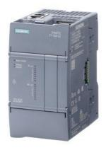
SIMATIC S7-1200 G2: failsafe compact CPU 1212FC DC/DC/DC; power supply: DC 20.4-28.8 V DC; onboard I/O: 8x DI 24 V DC; 6x DO 24 V DC; memory: program 200 KB data: 500 KB, retentivity: 20 KB
