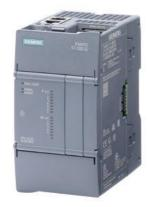
SIMATIC S7-1200 G2: compact CPU 1212C DC/DC/DC; power supply: DC 20.4-28.8 V DC; onboard I/O: 8x DI 24 V DC; 6x DO 24 V DC; memory: program 150 KB data: 500 KB, retentivity: 20 KB
