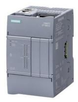
SIMATIC S7-1200 G2: failsafe compact CPU 1214FC DC/DC/DC; power supply: DC 20.4-28.8 V DC; onboard I/O: 14x DI 24 V DC; 10x DO 24 V DC; memory: program 300 KB data: 750 KB, retentivity: 20 KB
