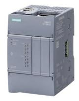
SIMATIC S7-1200 G2: compact CPU 1214C AC/DC/RLY; power supply: AC 85-264 V AC at 47-63 Hz; onboard I/O: 14x DI 24 V DC; 10 DO relay 2 A; memory: program 250 KB data: 750 KB, retentivity: 20 KB
