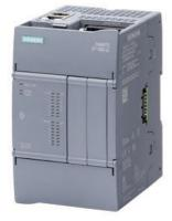
SIMATIC S7-1200 G2: compact CPU 1214C DC/DC/RLY; power supply: DC 20.4-28.8 V DC; onboard I/O: 14x DI 24 V DC; 10 DO relay 2 A; memory: program 250 KB data: 750 KB, retentivity: 20 KB
